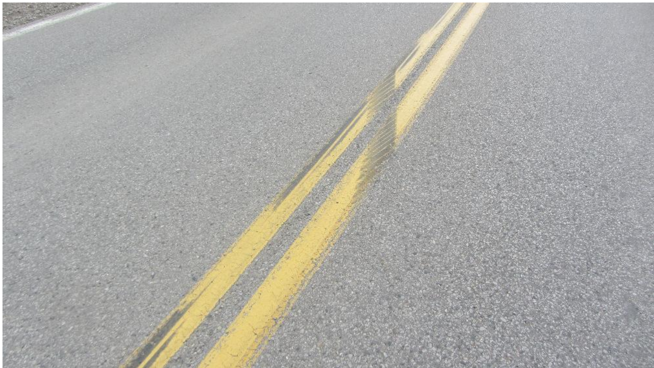
Figure 16: View of black yaw marks on the roadway centre-line.
