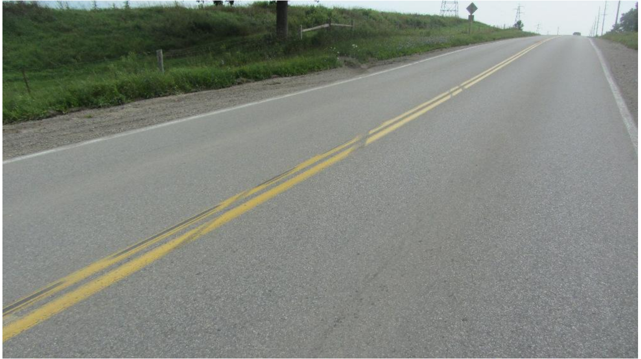
Figure 15: Looking north-east at the black yaw marks visible on the yellow centre-line.
